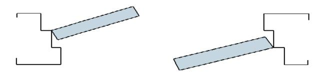
Type of Astragal? Flat or Z Type (Z astragal be on one door leaf only) Installed? Yes or No Method of install? Screw On (std) or Welded (optional) Tag # \_\_\_\_\_
