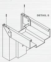
15) Secure or save glass bead for installation of glass and glazing
