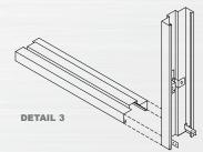
8) Fit top of vertical mullion over bracket in head (see detail 4)
