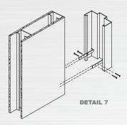
14) Install screws in corner gussets (see detail 8)
