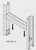
11) Finish tightening compression anchors in both jambs, alternating counter-clockwise turns of compression anchors to assure head remains square (see details 6 & B)
