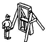
10. PLACE AND SUPPORT A WOOD SPREADER AT CENTER OF FRAME. SEE "STEP #4" FOR SIZE.
