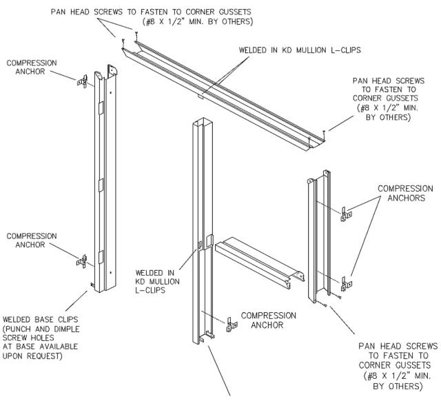
WELDED BASE CLIPS AT BLOWOUT. (PUNCH AND DIMPLE SCREW HOLES AT BASE AVAILABLE UPON REQUEST)
